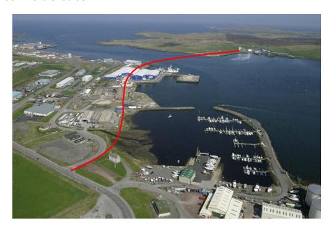
Option 2: High Level Bridge: This option covers a high level bridge with an airdraft of 60m above MHWS over a 260m wide channel. The bridge would also be provided with wind shielding. It would allow two directional traffic and
