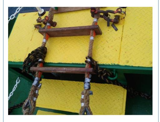
This image shows the secondary lashings after being requested by the Pilot. As per good seamanship these secondary lashing should be a
