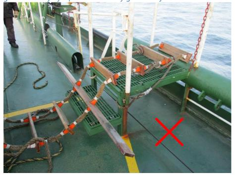
This also shows a secondary lashing spliced around a hard angle. This is not a dedicated securing point.
