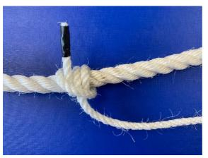
rolling hitch<sup>1</sup> with the standing part leading so that the lashing seizes when weight is applied to the ladder.
