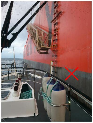
This image shows an accommodation ladder with a non-horizontal platform and a distance from the platform to sea level of less than 5m.
