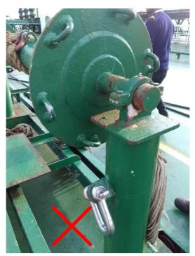
This example shows a winch reel that has not been mechanically secured.
