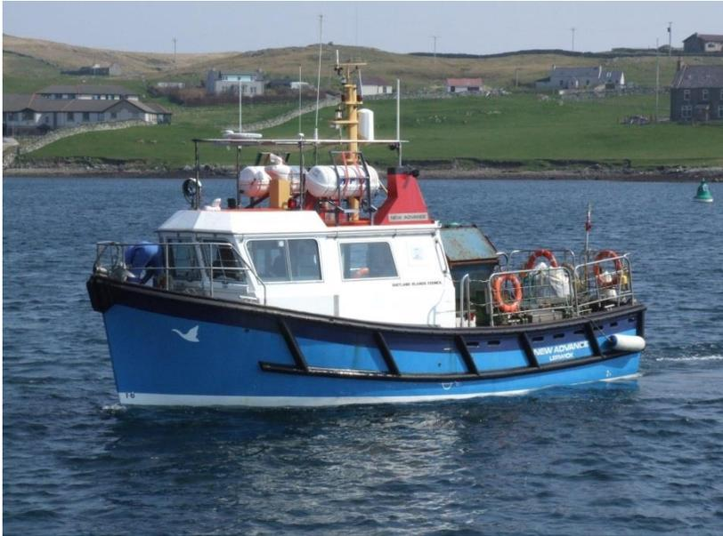
**Vessel Issues:** Vessel is relatively slow (8 knots) and has a very low carrying capacity.
