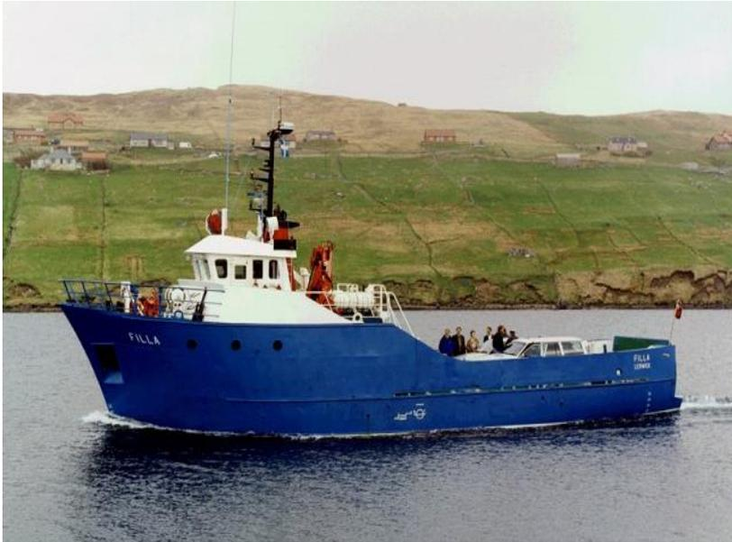
**Vessel Issues:** Vessel is single screwed; insufficient sub-division below the waterline; ageing vessel.
