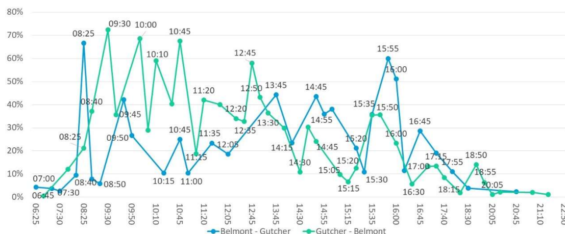
Figure 7.6: Proportion of Gutcher – Belmont route leg sailings in 2024 where vehicle deck utilisation exceeded 75% (Source: vessel logbooks)
