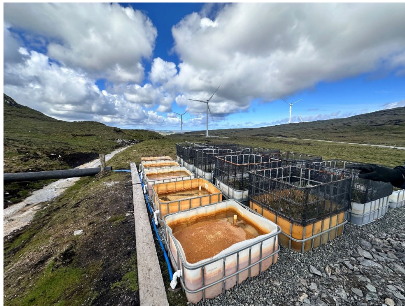
Photo 4. Pilot trials for new design of drainage treatment system at KBP02
