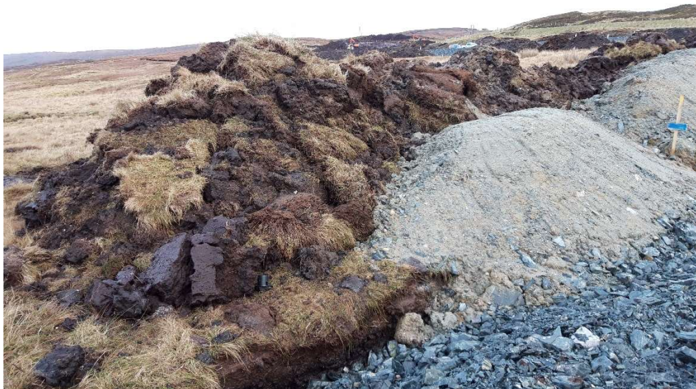
Photo 3. Turves and mineral soils observed at the western end of Sandwater Road.
