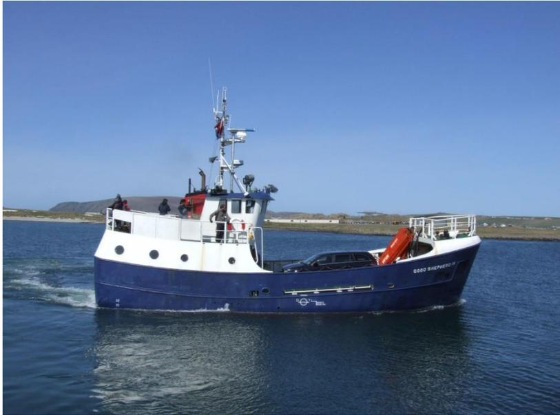
**Vessel Issues:** Vessel is relatively old, single screwed and slow (8 knots).
