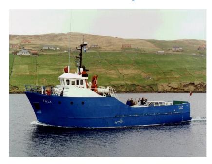
**Vessel Issues:** Vessel is single screwed; insufficient sub-division below the waterline; ageing vessel.
