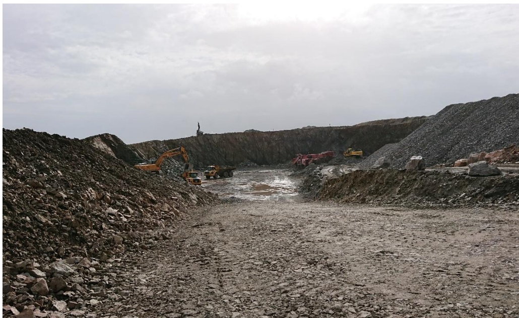
Photo 12. View of active rock extraction at NBP05, mobile crusher and screening plant for the production of aggregate can be seen.
