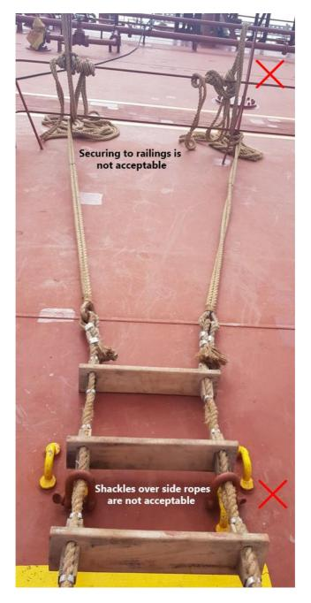
Sullom Voe <u>will not accept</u> Pilot Ladders secured around railings or hand rails.
