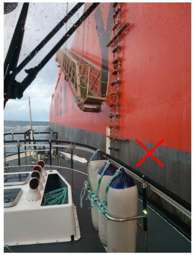
This image shows an accommodation ladder with a non-horizontal platform and a distance from the platform to sea level of less than 5m.
