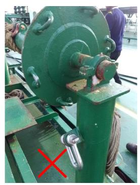
This example shows a winch reel that has not been mechanically secured.
