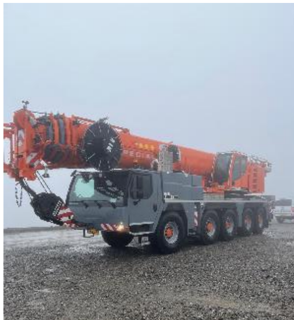
Photo 8. K43 – telescopic boom mobile crane
