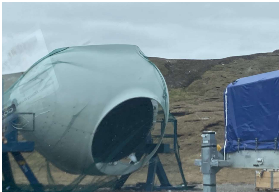
Photo 2. Netting placed over hub section and plastic wrapping covering holes of support frame as bird deterrents at T025
