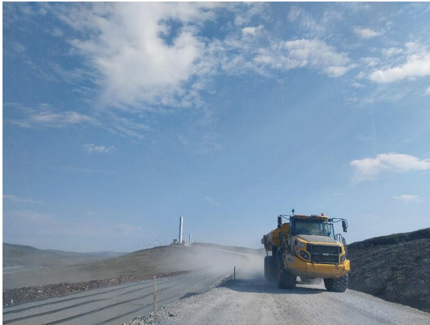
Photo 17. Articulated Dumper Truck (ADT) on road before dust suppression management activity
