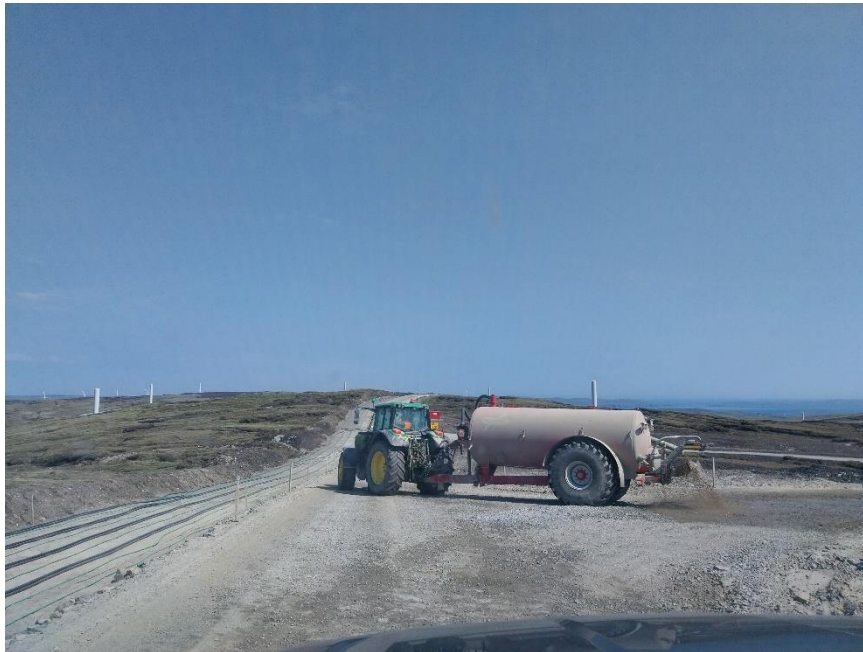
Photo 15. Bowser deployed on dust suppression activity by NBP05
