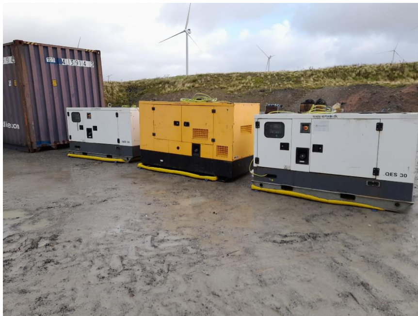
Photo 11. Plant nappies beneath generators in northern compound
